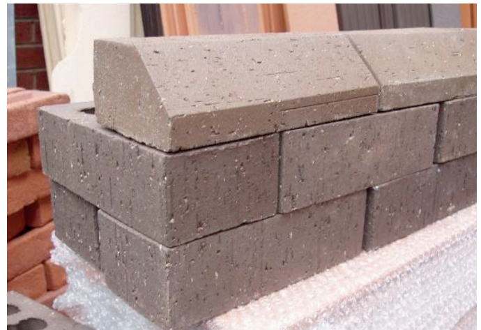
Due to different extrusion processes, the drag wire marks on the plinth bricks run horizontal whilst the standard bricks are vertical.
