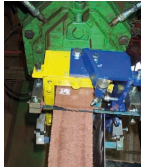
Column of extruded clay undergoing a rusticated texture.
