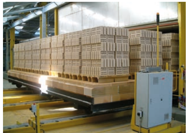
Kiln car exiting a tunnel kiln.
